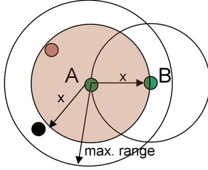
Figure 3.1: Minimal transmission power used during whispering between (green) nodes  $A$  and  $B$ . Attacker's node positioned inside the inner circle (red node) is able to eavesdrop the transmission between  $A$  and  $B$  whereas node positioned outside (black node) is not.
