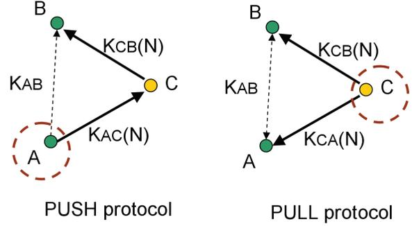
Figure 3.2: Graphic representation of the simplest version of Push and Pull amplification protocols with only one intermediate node  $C$ . Red dashed circle highlights the node generating a fresh new random secret  $N$ .  $K_{xy}$  is the existing directional key between nodes  $x$  and  $y$ .
