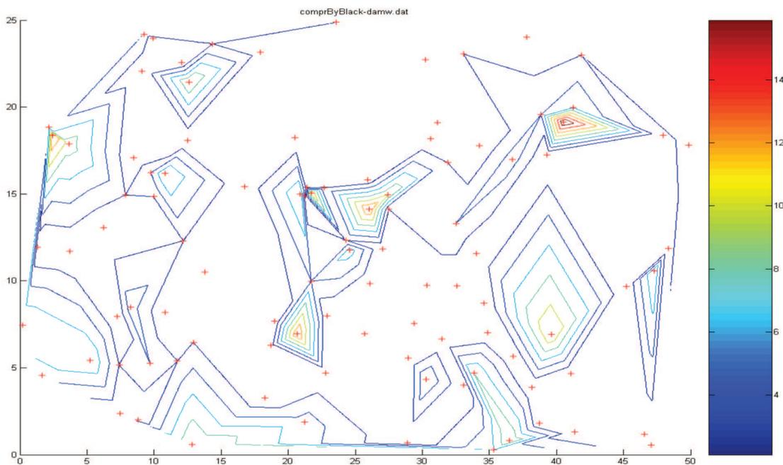
Figure 3.8: Example of non-uniform distribution of the link key compromise for the Pull protocol. Two-dimensional deployment plane is displayed with number of compromised link keys as third axis. Red crosses show position of the eavesdropping nodes. Legal nodes are not shown for the clarity reasons.
