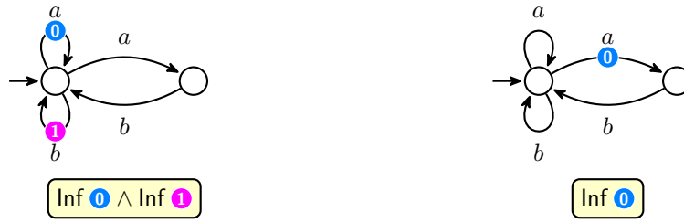
■ Figure 1 The left automaton accepts the words that contain infinitely many occurrences of both a and b . Each accepting run of the left automaton has to contain infinitely many occurrences of both transitions looping on the initial state. Hence, there does not exist any automaton with the same accepting runs as the left automaton and less than two acceptance marks. The right automaton accepts the same language using one acceptance mark and a different set of accepting runs.
