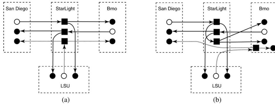
Fig. 2. Connection scheme for (a) the first and (b) the second iGrid experiment. The full lines show uncompressed HD streams; the dotted line shows compressed HDV streams. The empty circles denote sending computers, the full circles stand for display computers, and the full boxes are AEs.
