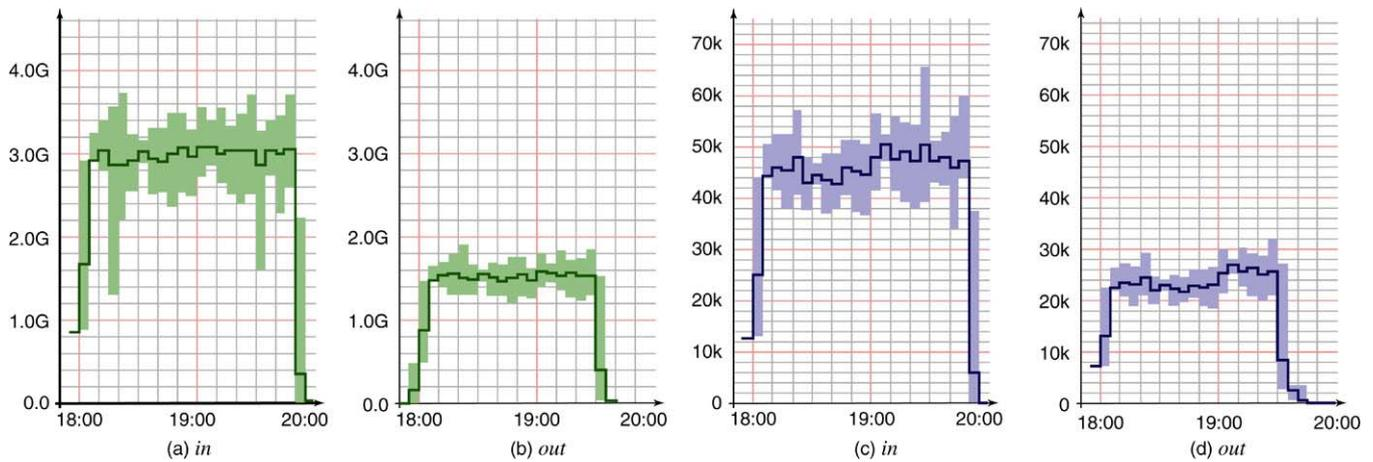
Fig. 3. Network statistics gathered on the Brno uplink. The lines are five minute averages, while the surface is an envelope curve with min/max values within the five minute interval. (a) gives *in* throughput in Gbps, (b) gives *out* throughput in Gbps, (c) gives *in* throughput in packets per second (pps), and (d) gives *out* throughput in pps.
