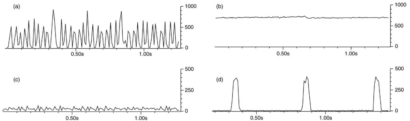
Fig. 4. Bursty traffic produced by the uncompressed HD transport (a) compared to smooth traffic by our measurement probes (b). Bursty traffic produced by the HDV transport with VLC (c) and net cat (d). Vertical axis denotes number of packets per 20 ms interval.
