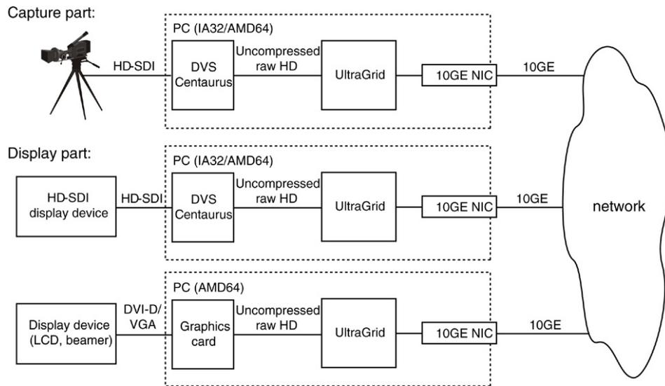
Fig. 1. Site connection scheme for HD transmission.
