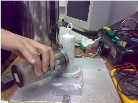
Figure 2.1: Freezing a smartcard chip by liquid nitrogen.
