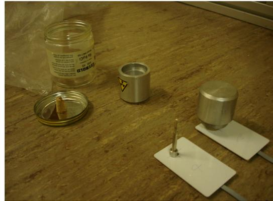
Figure 2.2: Unsealed sources emitting alpha and beta particles.
