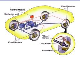
► The controller monitors the speed sensors in wheels Right before a wheel locks up, it experiences a rapid deceleration
