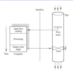
Computer controls the flow in the pipe in real-time
