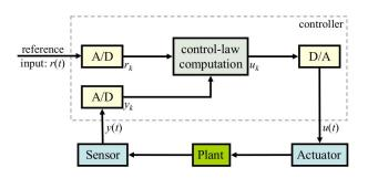
The controller (computer) controls the plant using the actuator (valve) based on sampled data from the sensor (flow meter)
