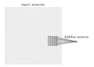
Every neuron is connected with a (typically small) *receptive field* of neurons in the lower layer.
