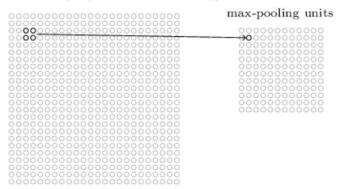
Neurons in the pooling layer compute simple functions of their receptive fields (the fields are typically disjoint):
