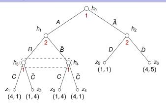
What we designate as subgames to allow the backward induction? Only subtrees rooted in  $h_1$ ,  $h_2$ , and  $h_0$  (together with all subtrees rooted in terminal nodes)
