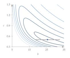
The engineers would refuse the solution: The aspect ratio is much higher than typically seen in airplanes. It adversely affects the structural strength. Add constraints!
