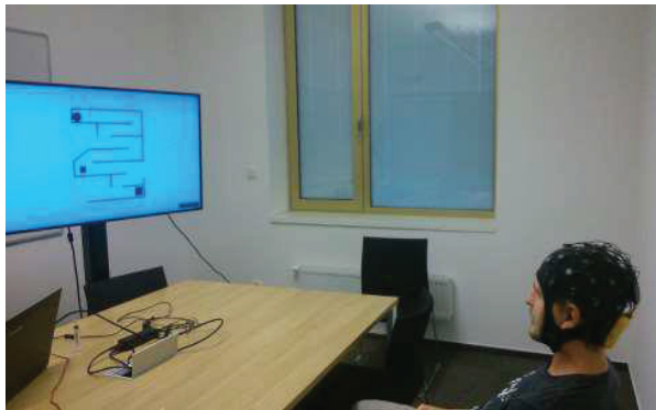
Fig. 1. Experimental setup. Left: the game feedback. Right: participant during game control through the BCI.
