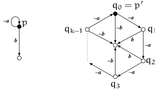
In this picture, each node  $q_i$  has an outgoing edge going to a “dead” state; this edge is labelled  $b$  if  $i \in J$  and labelled  $-b$  if  $i \notin J$ . It is straightforward to check that the proposed implementation of  $R_J(x)$  is indeed correct.
