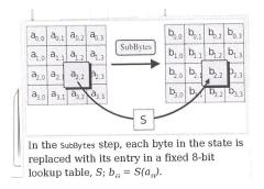
In this step, each byte in the state is replaced with its entry in a fixed 8-bit lookup table.
