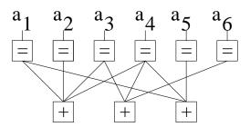
The corresponding parity check matrix has n-k rows and n columns and i-th column has 1 in the j-th row exactly in case if i-th v-node is connected to j-th c-node.
