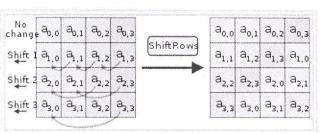
In the ShiftRows step, bytes in each row of the state are shifted cyclically to the left. The number of places each byte is shifted differs for each row.
