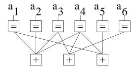
The corresponding parity check matrix has n-k rows and n columns and i-th column has 1 in the j-th row exactly in case if i-th v-node is connected to j-th v-node.
