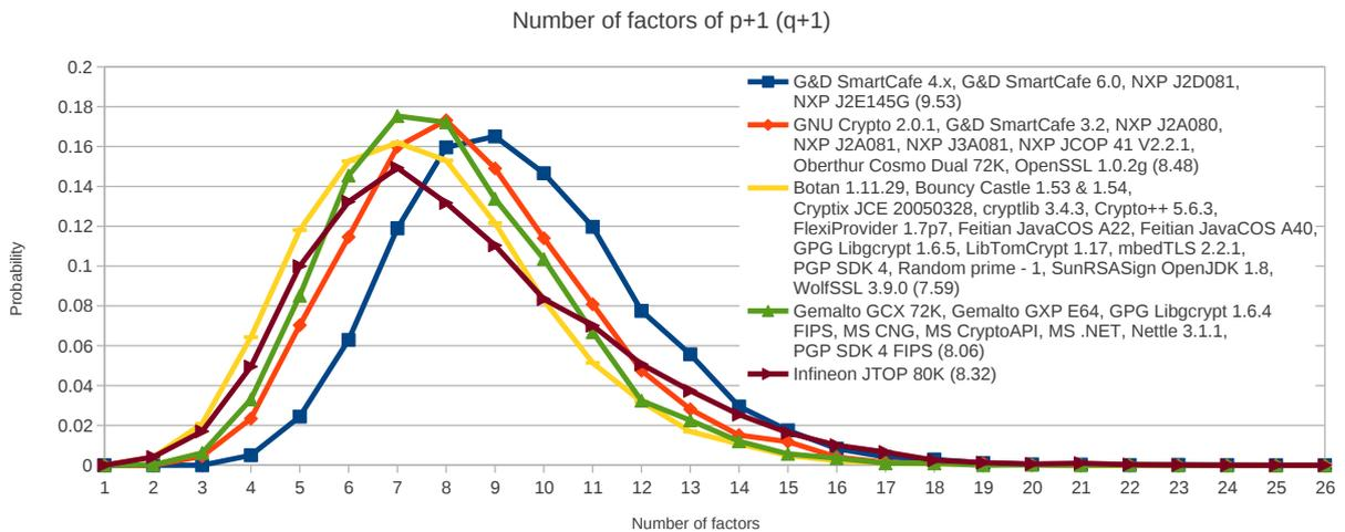
Figure 16: Number of factors of  $p + 1$  for RSA 512 bits. Histogram is generated from 10 000 factorized values of  $p + 1$  and  $q + 1$  taken from 5 000 key pairs. The sources behave more consistently, with only 5 distinguishable categories observed.
