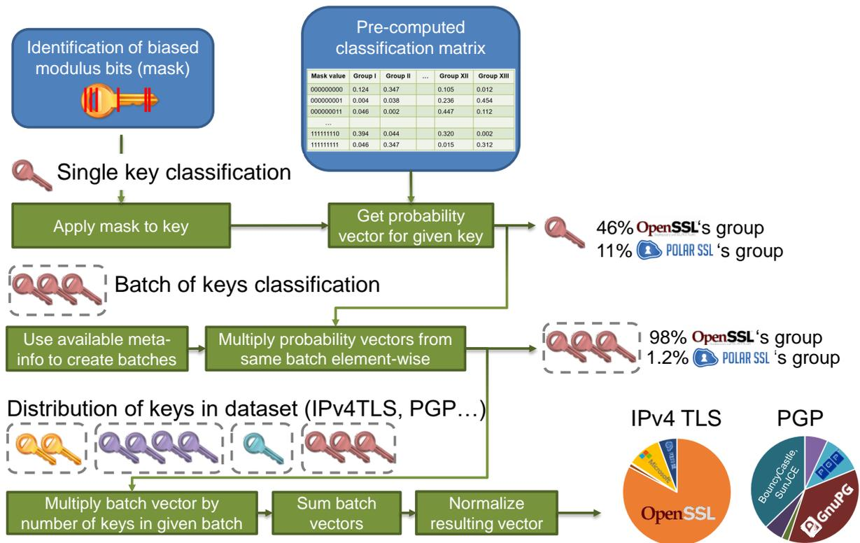
Figure 21: An example of the second phase of classification. Either a) single key, b) batch of keys from the same source or c) whole dataset of batches is classified using pre-computed classification matrix.
