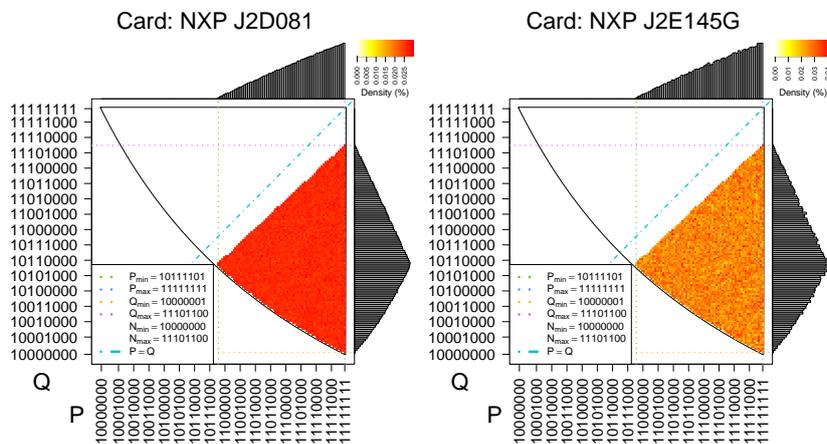
Figure 8: Cards: possibly rejection sampling. The primes generated by NXP J2D081 and NXP J2E145G are sorted and generated almost from the maximal region defined by modulus and prime bit lengths. Additionally, some requirement is placed on the difference of the primes. We hypothesize that the distribution can be easily reproduced by rejection sampling. See Figure 3 for the graph interpretation.
