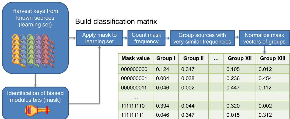
Figure 20: The first phase of classification of the RSA public keys. The groups of similar sources are established based on the statistical properties of a large number of keypairs generated by separate sources. As a result, a fixed classification matrix is pre-computed.
