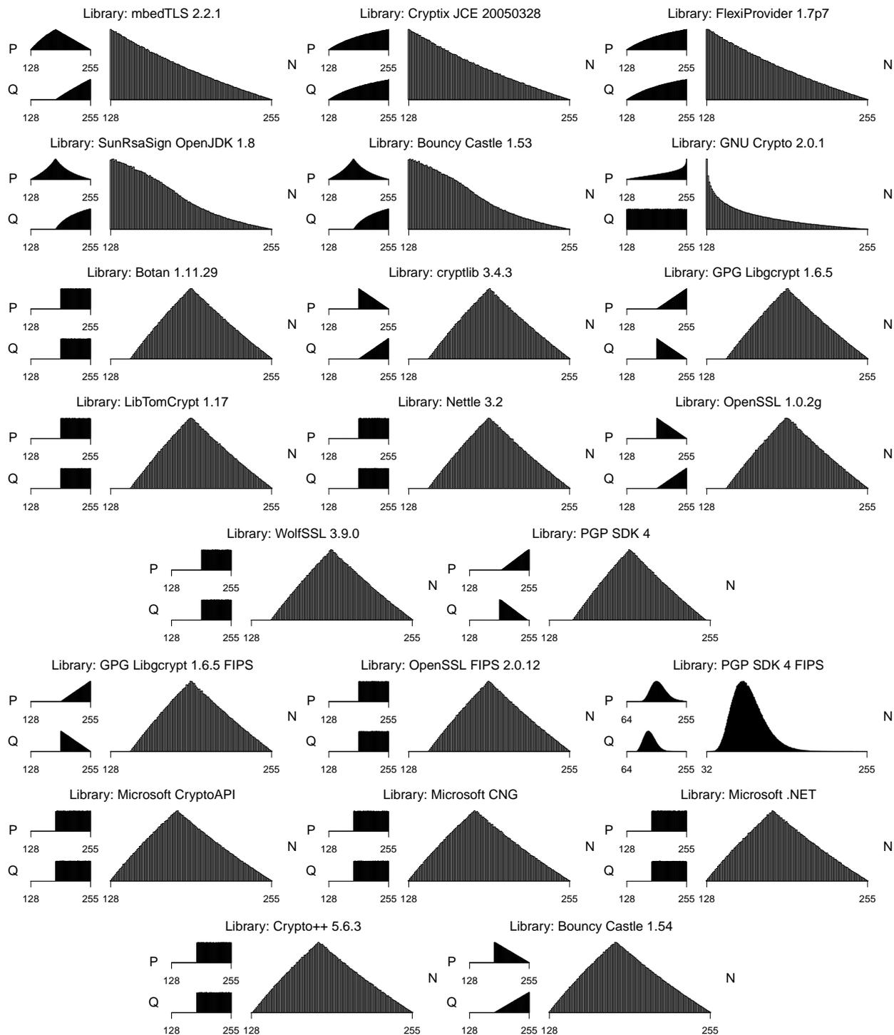
Figure 12: *Software libraries: the effect of distribution of the MSB of primes on the distribution of the MSB of the modulus.*
