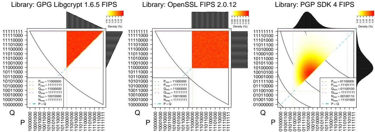
Figure 5: Libraries: FIPS variants. Libcrypt 1.6.5 in FIPS mode and OpenSSL FIPS module 2.0.12 generate strong primes uniformly and target the practical square region. PGP SDK 4 in FIPS mode generate strong primes from a different distribution. The primes may be one bit shorter than expected (notice the different values at the axes). As a result, the modulus may be shorter than requested, by one or two bits. See Figure 3 for the graph interpretation.
