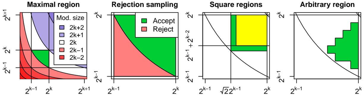
Figure 2: RSA key generation. The maximal region for the generated primes is defined by the precise length of the modulus and equal lengths of the primes. Such keys can be generated through rejection sampling. To avoid generating short moduli (which must be discarded), alternative square regions may be used. Several implementations, such as that of the NXP J2A080 card, generate primes from arbitrary combinations of square regions.
