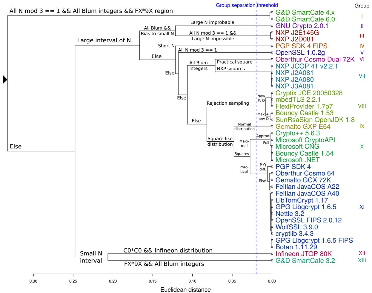
Figure 19: Annotated version of Figure 18. The reasons for the clustering and the computed Euclidean distances of mask values can be traced back to differences in the implementations.
