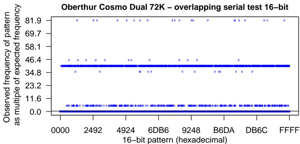
Figure 24: The frequencies of different patterns with the length of 16 bits computed from 2 MB random data stream generated by the Oberthur Cosmo Dual 72K card. Multiple distinct groups of patterns can be identified with some patterns never occurring in the tested random stream where patterns should be uniformly distributed instead.
