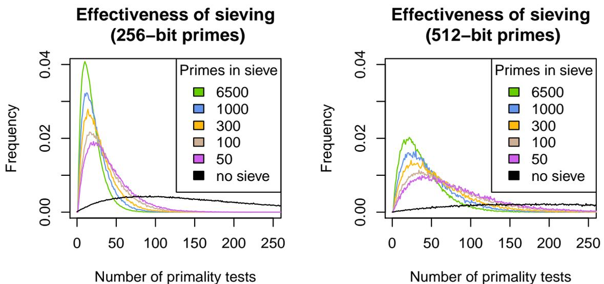
Figure 27: Trial division (or sieving) by a different number of small primes. Testing a candidate with division by a few primes decreases the number of required probabilistic primality tests and speeds up prime generation. The expected number of primality tests decreases when sieving phase runs with more primes.
