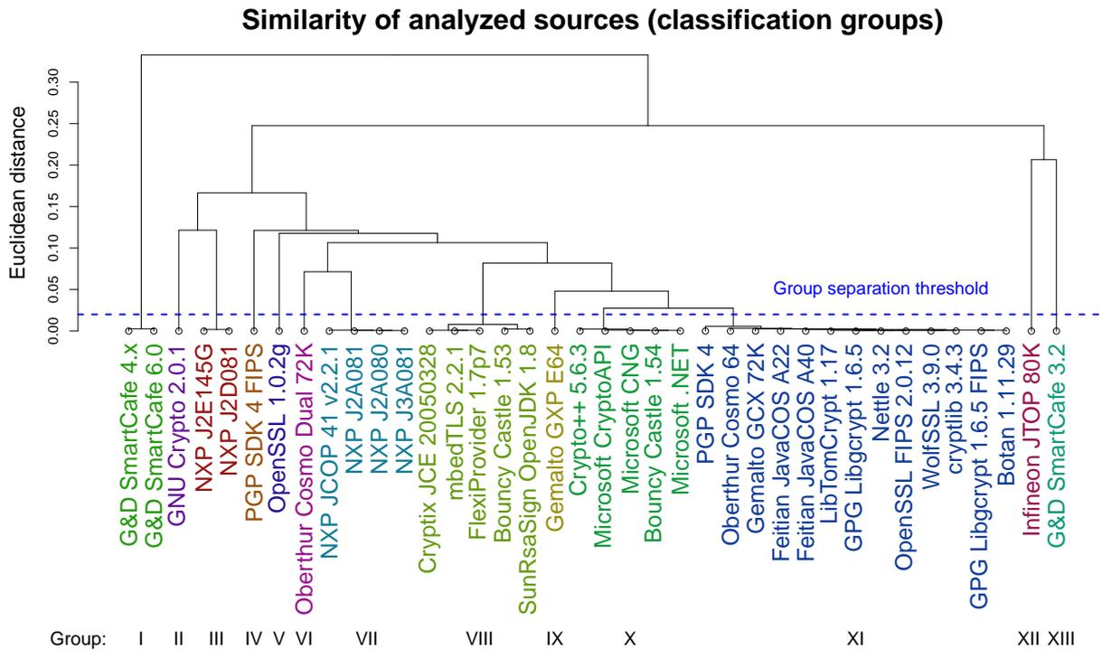
Figure 18: Clustering of all inspected sources based on the 9 bits of the mask. The separation line shows which sources were put by us into the same classification category. Finer separation is still possible (e.g., SunRsaSign vs mbedTLS), but the number of the keys from same source needs to be high enough to distinguish these very similar sources.
