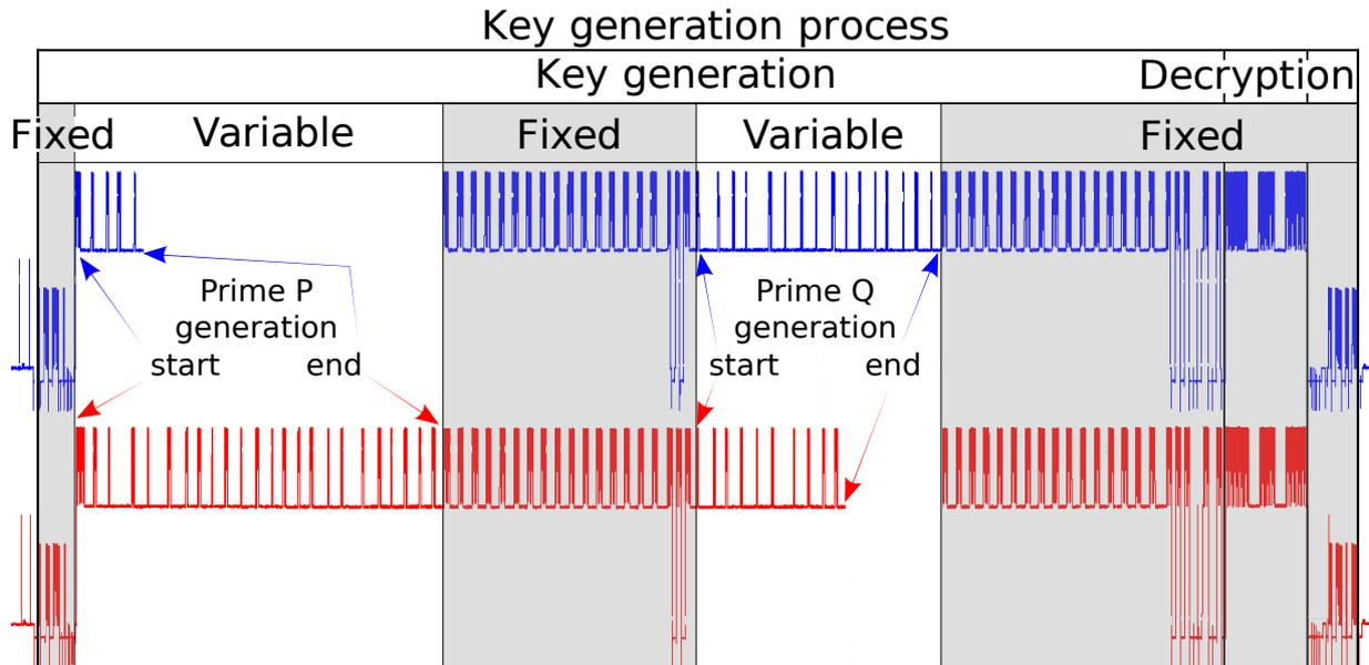
Figure 29: Annotated example power traces showing typical steps of on-card key pair generation. The upper trace is shorter in the first variable part (potentially corresponding to generation of first prime and longer in the second variable part). Both traces are intentionally interrupted to visually synchronize at fixed parts.
