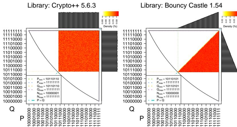
Figure 6: Libraries: the maximal square region. In the case of Crypto++ 5.6.3, the interval for prime generation is approximated. Bouncy Castle 1.54 generates primes from the truly maximal square region (besides ordering the primes afterwards). See Figure 3 for the graph interpretation.
