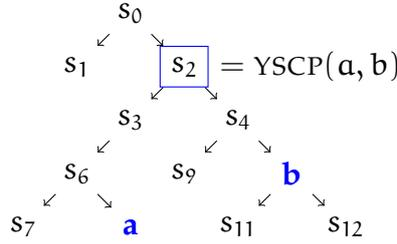
Figure 2:  $s_2$  is the Youngest State of the Common Path of a and b
