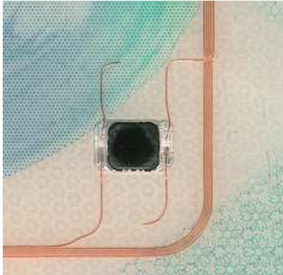
Fig. 1: Contactless chip and antenna from British passports.
