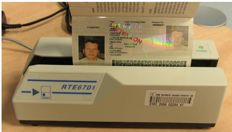
Fig. 2: Scanning of the machine-readable zone data.
