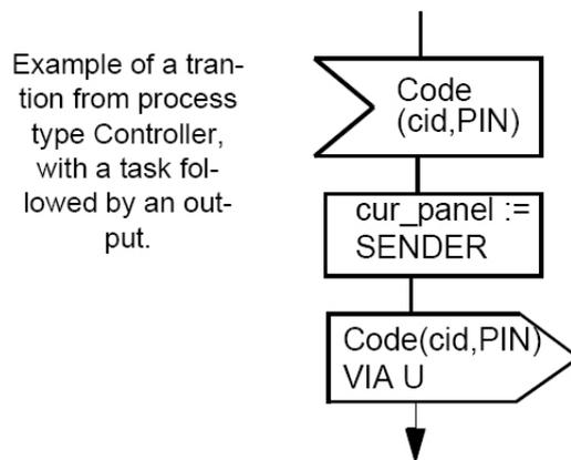
Figure 25: Finite State Machine
