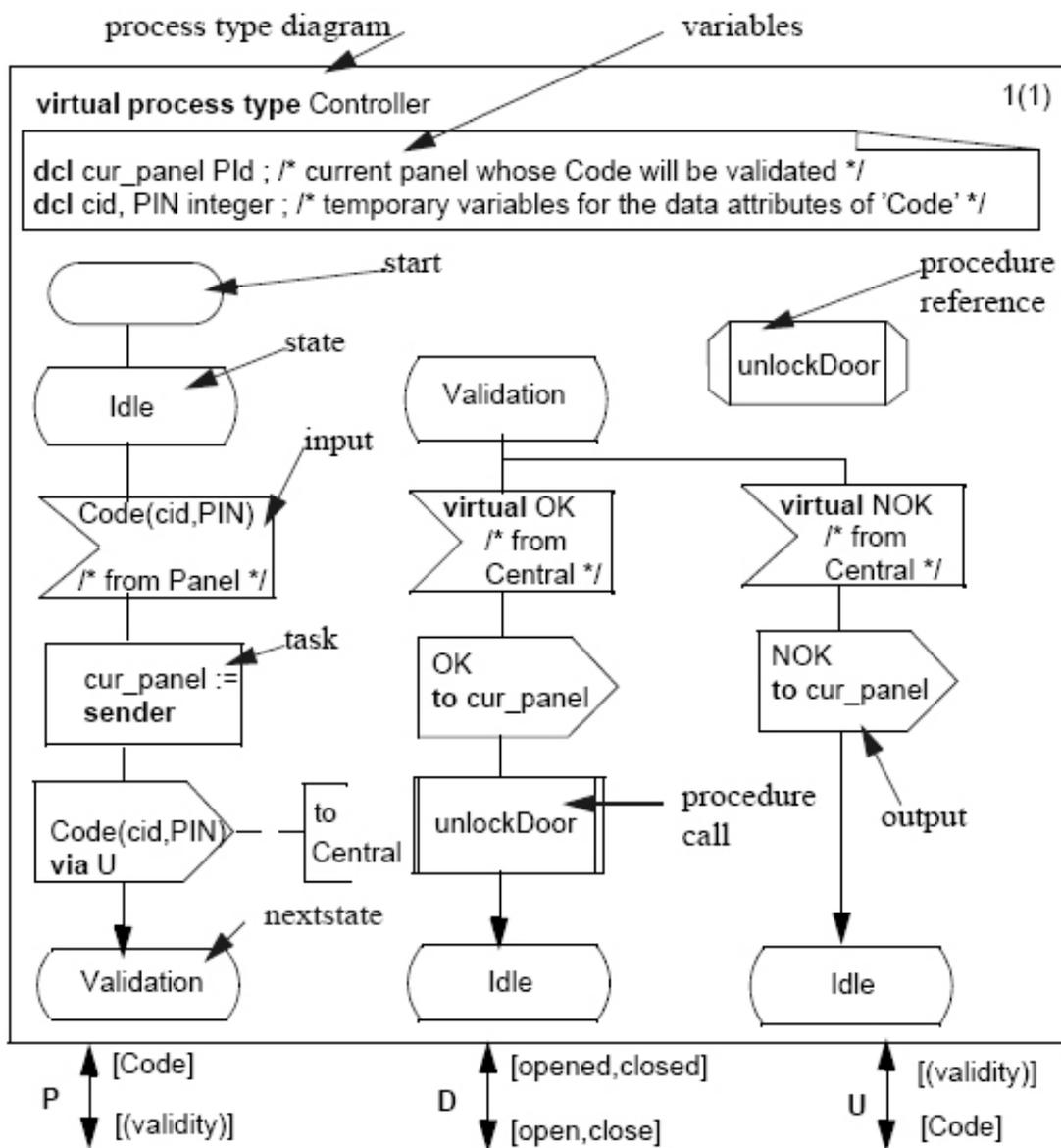
Figure 27: Finite State Machine of a process type
