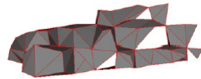
Figure 15: Uniform Vertex Clustering . 262 face approximation ( 11 \times 4 \times 4 grid). Indiscriminate joining destroys approximation quality.
