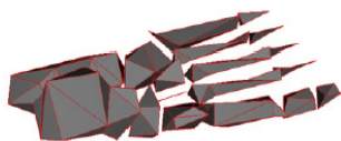
Figure 16: Edge Contractions . 250 face approximation. Bone segments at the ends of the toes have disappeared; the toes appear to be receding back into the foot.
