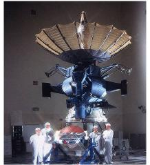
At the very beginning of the Galileo mission to explore Jupiter and its moons in 1989 it was discovered that primary antenna (deployed in the figure on the top) failed to deploy
