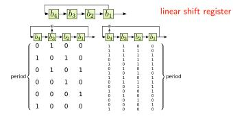
Theorem For every n > 0 there is a linear shift register of maximal period  $2^n - 1$ .
