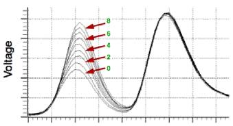
Hamming Weight or Hamming Distance Leakage
