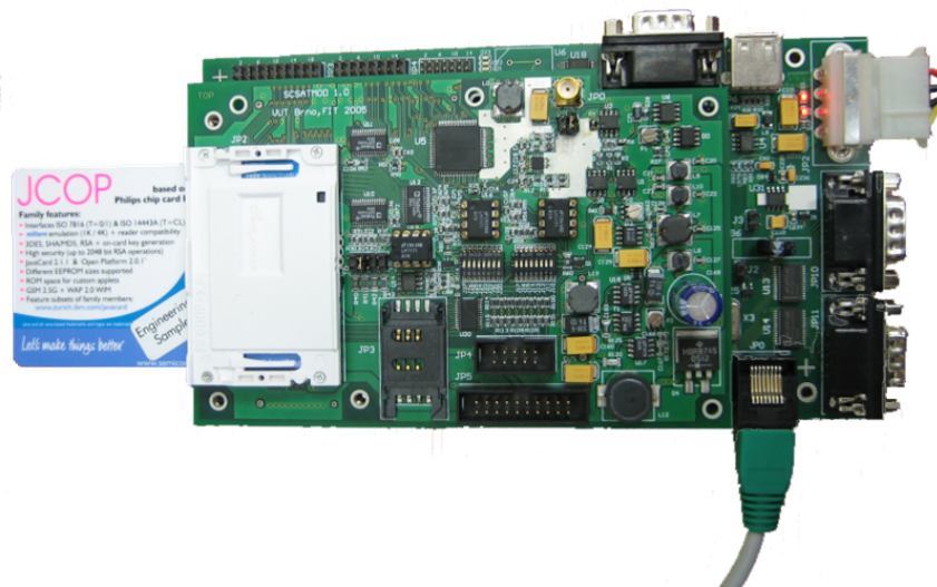
Figure 1: SCSAT04 power measurement device for cryptographic smart card analysis.
