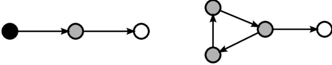
Figure 1 An example of possible cycle in solution. Black node is a producer, gray ones are distributors, and producers are the white ones.
